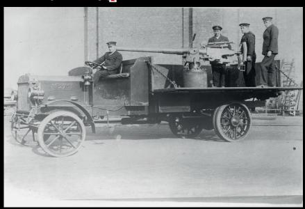
QF 3-pounder Vickers - Maxim (47 mm / L50) on the Mk I machine, cylindrical type.
